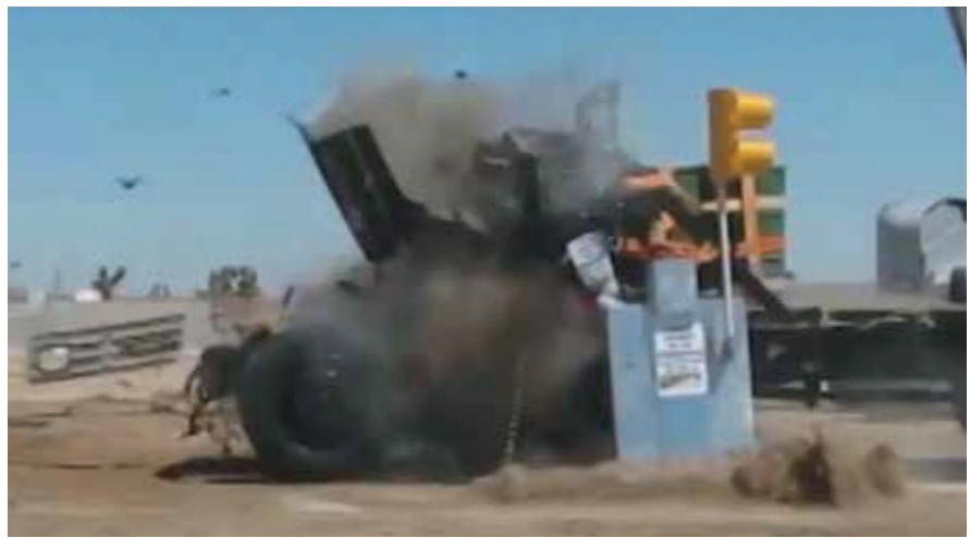
This video frame shows the moment of impact in a crash test. The front of the 15,000-lb truck moving at 30 MPH is cut apart by the barrier arm, but the bed of the truck (where the explosives would be) does not penetrate past the perimeter line.
