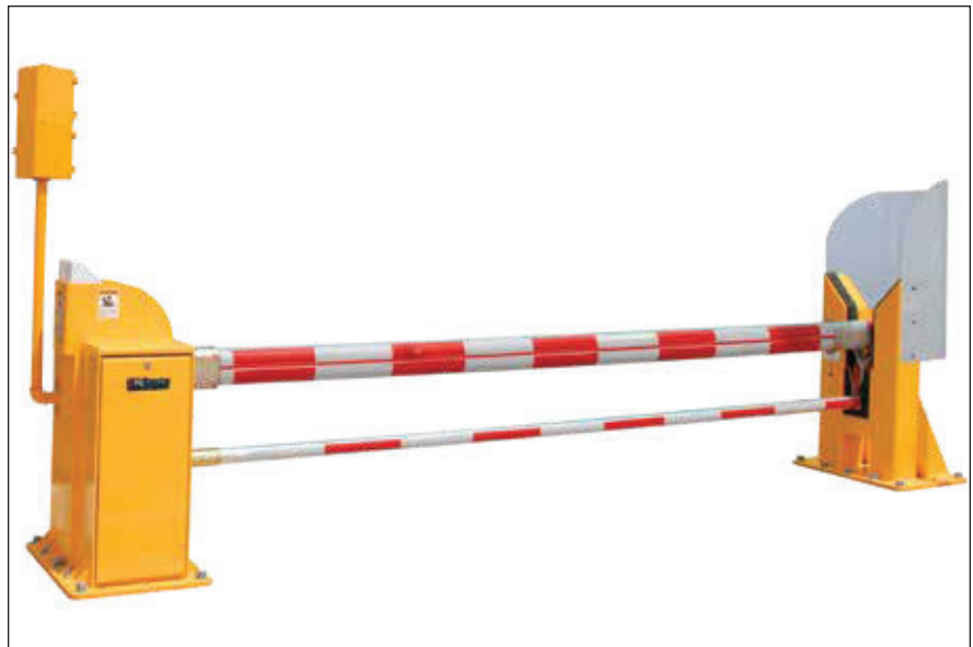
This crash-rated gate arm has a main barrier arm at the proper height to stop a 15,000-lb. truck, and a lower secondary arm added to prevent accidental crashes by shorter passenger vehicles, which could be fatal if the car’s windshield crashed into the truck-height barrier. IMAGE COURTESY OF HYSECURITY
